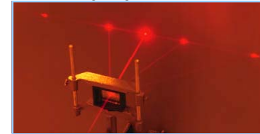
Diffraction grating and helium-neon laser
