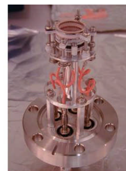
Figure 3; An example of the total fluorescence yield analyzer using MCP.
